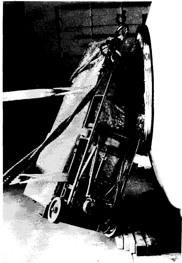
Fig. 1. MRI magnetic incompatibility. Ferromagnetic components within this radio-frequency power amplifier became magnetized when it was inadvertently moved too close to a 1.5 T superconducting magnet and the magnetic forces overcame the ability of the workmen moving the power supply to restrain it. A block and tackle apparatus was required to remove it from the magnet bore and the incident caused a magnet quench. (Photograph courtesy of Dr. W. A. Edelstein.)
