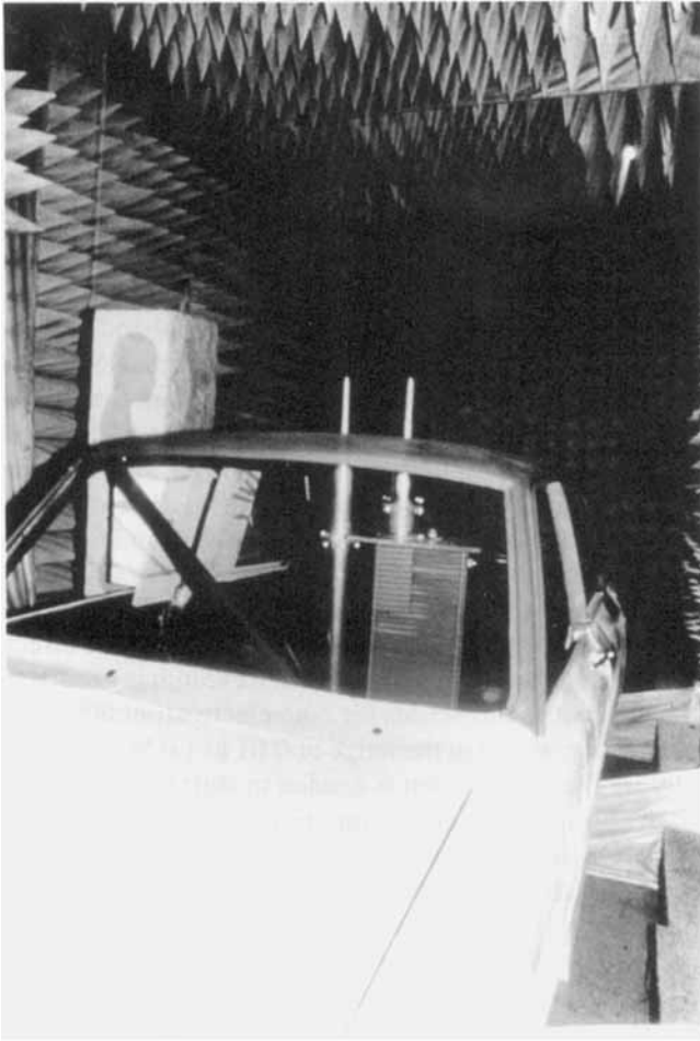
Fig. 3. Photograph showing a full-sized woman model (sagittal one-half) exposed to high-power (10 kW) mobile antenna fields in an anechoic chamber for the quantification of energy absorption.
