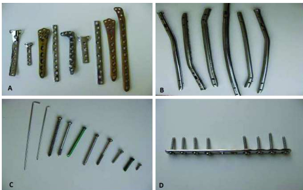
Fig. 4. Different types of removed metallic implants. (A) Plates (stainless steel and titanium), (B) intramedullary nails (stainless steel), (C) screws and pins (stainless steel and titanium) and, (D) an example of a plate with 8 screws (stainless steel) after removal from the site of implantation in the body.
