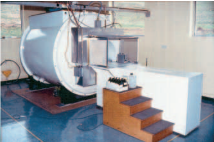
Figure 1. Photograph of home built magnetic resonance imager based on a 0.5 T super-conductive magnet.
